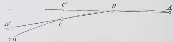
Fig. 22.—LAYING OUT A CURVE.
